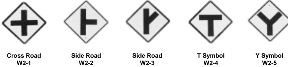
Figure 3. Intersection Warning Signs
